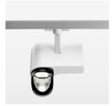
Surface-mounted luminaire with LED, rated life of the LED L80/B10 > 50000 h, chromaticity tolerance 2 SDCM (initial), reflector with asymmetrical light distribution pattern, primary reflector and kick reflector 99% pure aluminium in MIRO-Silver®, attachment with kick reflector to the ceiling approach of the light cone, exchangeable reflector unit in high-sheen black plastic, with glass cover, rotation angle 330°, swivel angle 90°, luminaire housing die-cast aluminium, powder-coated, stratowhite
