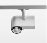
Surface-mounted luminaire with LED, rated life of the LED L80/B10 > 50000 h, colour rendering index CRI > 96, chromaticity tolerance 3 SDCM (initial), , reflector with circular light distribution pattern, reflector pure aluminium 99,99% in MIRO-Silver®, segmented and faceted, exchangeable reflector unit in high-sheen black plastic, with glass cover, rotation angle 330°, swivel angle 90°, luminaire housing die-cast aluminium, powder-coated, stratosilver
