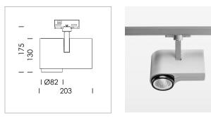
Surface-mounted luminaire with LED, rated life of the LED L80/B10 > 50000 h, chromaticity tolerance 3 SDCM (initial), , reflector with circular light distribution pattern, reflector pure aluminium 99,99% in MIRO-Silver®, segmented and faceted, exchangeable reflector unit in high-sheen black plastic, with glass cover, rotation angle 330°, swivel angle 90°, luminaire housing diecast aluminium, powder-coated, stratosilver
