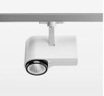
Surface-mounted luminaire with LED, rated life of the LED L80/B10 > 50000 h, colour rendering index CRI > 90, chromaticity tolerance 2 SDCM (initial), , reflector with circular light distribution pattern, reflector pure aluminium 99,99% in MIRO-Silver®, segmented and faceted, exchangeable reflector unit in high-sheen black plastic, with glass cover, rotation angle 330°, swivel angle 90°, luminaire housing die-cast aluminium, powder-coated, stratowhite
