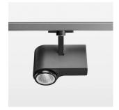
Surface-mounted luminaire with LED, rated life of the LED L80/B10 > 50000 h, colour rendering index CRI > 80, chromaticity tolerance 2 SDCM (initial), reflector with circular light distribution pattern, reflector pure aluminium 99,99% in MIRO-Silver®, segmented and faceted, exchangeable reflector unit in high-sheen black plastic, with glass cover, rotation angle 330°, swivel angle 90°, luminaire housing die-cast aluminium, powder-coated, stratoblack
