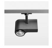
Surface-mounted luminaire with LED, rated life of the LED L80/B10 > 50000 h, chromaticity tolerance 3 SDCM (initial), , reflector with circular light distribution pattern, reflector pure aluminium 99,99% in MIRO-Silver®, segmented and faceted, exchangeable reflector unit in high-sheen black plastic, with glass cover, rotation angle 330°, swivel angle 90°, luminaire housing diecast aluminium, powder-coated, stratoblack
