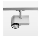
Surface-mounted luminaire with LED, rated life of the LED L80/B10 > 50000 h, colour rendering index CRI > 80, chromaticity tolerance 2 SDCM (initial), reflector with circular light distribution pattern, reflector pure aluminium 99,99% in MIRO-Silver®, segmented and faceted, exchangeable reflector unit in high-sheen black plastic, with glass cover, rotation angle 330°, swivel angle 90°, luminaire housing die-cast aluminium, powder-coated, stratosilver
