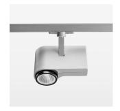
Surface-mounted luminaire with LED, rated life of the LED L80/B10 > 50000 h, chromaticity tolerance 3 SDCM (initial), , reflector with circular light distribution pattern, reflector pure aluminium 99,99% in MIRO-Silver®, segmented and faceted, exchangeable reflector unit in high-sheen black plastic, with glass cover, rotation angle 330°, swivel angle 90°, luminaire housing diecast aluminium, powder-coated, stratosilver
