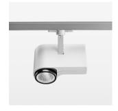
Surface-mounted luminaire with LED, rated life of the LED L80/B10 > 50000 h, colour rendering index CRI > 90, chromaticity tolerance 2 SDCM (initial), reflector with circular light distribution pattern, reflector pure aluminium 99,99% in MIRO-Silver®, segmented and faceted, exchangeable reflector unit in high-sheen black plastic, with glass cover, rotation angle 330°, swivel angle 90°, luminaire housing die-cast aluminium, powder-coated, stratowhite
