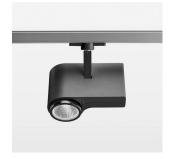
Surface-mounted luminaire with LED, rated life of the LED L80/B10 > 50000 h, colour rendering index CRI > 96, chromaticity tolerance 2 SDCM (initial), reflector with circular light distribution pattern, reflector pure aluminium 99,99% in MIRO-Silver®, segmented and faceted, exchangeable reflector unit in high-sheen black plastic, with glass cover, rotation angle 330°, swivel angle 90°, luminaire housing die-cast aluminium, powder-coated, stratoblack
