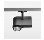
Surface-mounted luminaire with LED, rated life of the LED L80/B10 > 50000 h, colour rendering index CRI > 96, chromaticity tolerance 3 SDCM (initial), reflector with circular light distribution pattern, reflector pure aluminium 99,99% in MIRO-Silver®, segmented and faceted, exchangeable reflector unit in high-sheen black plastic, with glass cover, rotation angle 330°, swivel angle 90°, luminaire housing die-cast aluminium, powder-coated, stratoblack
