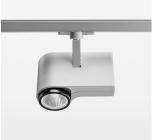
Surface-mounted luminaire with LED, rated life of the LED L80/B10 > 50000 h, colour rendering index CRI > 80, chromaticity tolerance 2 SDCM (initial), , reflector with circular light distribution pattern, reflector pure aluminium 99,99% in MIRO-Silver®, segmented and faceted, exchangeable reflector unit in high-sheen black plastic, with glass cover, rotation angle 330°, swivel angle 90°, luminaire housing die-cast aluminium, powder-coated, stratosilver
