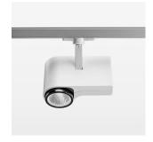
Surface-mounted luminaire with LED, rated life of the LED L80/B10 > 50000 h, colour rendering index CRI > 96, chromaticity tolerance 2 SDCM (initial), reflector with circular light distribution pattern, reflector pure aluminium 99,99% in MIRO-Silver®, segmented and faceted, exchangeable reflector unit in high-sheen black plastic, with glass cover, rotation angle 330°, swivel angle 90°, luminaire housing die-cast aluminium, powder-coated, stratowhite
