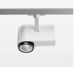
Surface-mounted luminaire with LED, rated life of the LED L80/B10 > 50000 h, colour rendering index CRI > 96, chromaticity tolerance 3 SDCM (initial), , reflector with circular light distribution pattern, reflector pure aluminium 99,99% in MIRO-Silver®, segmented and faceted, exchangeable reflector unit in high-sheen black plastic, with glass cover, rotation angle 330°, swivel angle 90°, luminaire housing die-cast aluminium, powder-coated, stratowhite
