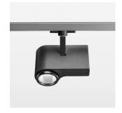
Surface-mounted luminaire with LED, rated life of the LED L80/B10 > 50000 h, chromaticity tolerance 2 SDCM (initial), LED hybrid technology, 3D silicone lens to reduce the proportion of scattered light, reflector with oval light distribution pattern, reflector pure aluminium 99,99% in MIRO-Silver®, segmented, exchangeable reflector unit in high-sheen black plastic, with glass cover, rotation angle 330°, swivel angle 90°, luminaire housing die-cast aluminium, powder-coated, stratoblack
