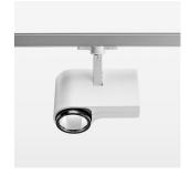
Surface-mounted luminaire with LED, rated life of the LED L80/B10 > 50000 h, chromaticity tolerance 2 SDCM (initial), LED hybrid technology, 3D silicone lens to reduce the proportion of scattered light, reflector with oval light distribution pattern, reflector pure aluminium 99,99% in MIRO-Silver®, segmented, exchangeable reflector unit in high-sheen black plastic, with glass cover, rotation angle 330°, swivel angle 90°, luminaire housing die-cast aluminium, powder-coated, stratowhite
