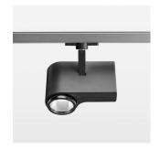
Surface-mounted luminaire with LED, rated life of the LED L80/B10 > 50000 h, chromaticity tolerance 2 SDCM (initial), LED hybrid technology, 3D silicone lens to reduce the proportion of scattered light, reflector with oval light distribution pattern, reflector pure aluminium 99,99% in MIRO-Silver®, segmented, exchangeable reflector unit in high-sheen black plastic, with glass cover, rotation angle 330°, swivel angle 90°, luminaire housing die-cast aluminium, powder-coated, stratoblack
