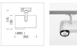
Surface-mounted luminaire with LED, rated life of the LED L80/B10 > 50000 h, chromaticity tolerance 2 SDCM (initial), LED hybrid technology, 3D silicone lens to reduce the proportion of scattered light, reflector with oval light distribution pattern, reflector pure aluminium 99,99% in MIRO-Silver®, segmented, exchangeable reflector unit in high-sheen black plastic, with glass cover, rotation angle 330°, swivel angle 90°, luminaire housing die-cast aluminium, powder-coated, stratowhite
