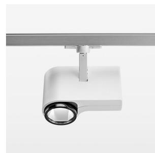
Surface-mounted luminaire with LED, rated life of the LED L80/B10 > 50000 h, chromaticity tolerance 3 SDCM (initial), LED hybrid technology, 3D silicone lens to reduce the proportion of scattered light, reflector with oval light distribution pattern, reflector pure aluminium 99,99% in MIRO-Silver®, segmented, exchangeable reflector unit in high-sheen black plastic, with glass cover, rotation angle 330°, swivel angle 90°, luminaire housing die-cast aluminium, powder-coated, stratowhite
