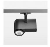
Surface-mounted luminaire with LED, rated life of the LED L80/B10 > 50000 h, chromaticity tolerance 3 SDCM (initial), LED hybrid technology, 3D silicone lens to reduce the proportion of scattered light, reflector with oval light distribution pattern, reflector pure aluminium 99,99% in MIRO-Silver®, segmented, exchangeable reflector unit in high-sheen black plastic, with glass cover, rotation angle 330°, swivel angle 90°, luminaire housing die-cast aluminium, powder-coated, stratoblack
