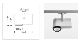
Surface-mounted luminaire with LED, rated life of the LED L80/B10 > 50000 h, chromaticity tolerance 3 SDCM (initial), LED hybrid technology, 3D silicone lens to reduce the proportion of scattered light, reflector with oval light distribution pattern, reflector pure aluminium 99,99% in MIRO-Silver®, segmented, exchangeable reflector unit in high-sheen black plastic, with glass cover, rotation angle 330°, swivel angle 90°, luminaire housing die-cast aluminium, powder-coated, stratosilver
