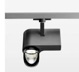
Surface-mounted luminaire with LED, rated life of the LED L80/B10 > 50000 h, chromaticity tolerance 2 SDCM (initial), reflector with asymmetrical light distribution pattern, primary reflector and kick reflector 99% pure aluminium in MIRO-Silver®, attachment with kick reflector to the ceiling approach of the light cone, exchangeable reflector unit in high-sheen black plastic, with glass cover, rotation angle 330°, swivel angle 90°, luminaire housing die-cast aluminium, powder-coated, stratoblack
