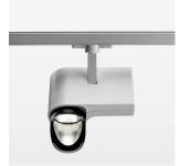
Surface-mounted luminaire with LED, rated life of the LED L80/B10 > 50000 h, chromaticity tolerance 2 SDCM (initial), reflector with asymmetrical light distribution pattern, primary reflector and kick reflector 99% pure aluminium in MIRO-Silver®, attachment with kick reflector to the ceiling approach of the light cone, exchangeable reflector unit in high-sheen black plastic, with glass cover, rotation angle 330°, swivel angle 90°, luminaire housing die-cast aluminium, powder-coated, stratosilver
