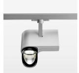
Surface-mounted luminaire with LED, rated life of the LED L80/B10 > 50000 h, chromaticity tolerance 3 SDCM (initial), reflector with asymmetrical light distribution pattern, primary reflector and kick reflector 99% pure aluminium in MIRO-Silver®, attachment with kick reflector to the ceiling approach of the light cone, exchangeable reflector unit in high-sheen black plastic, with glass cover, rotation angle 330°, swivel angle 90°, luminaire housing die-cast aluminium, powder-coated, stratosilver
