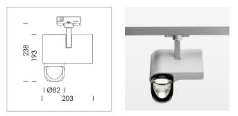
Surface-mounted luminaire with LED, rated life of the LED L80/B10 > 50000 h, chromaticity tolerance 3 SDCM (initial), reflector with asymmetrical light distribution pattern, primary reflector and kick reflector 99% pure aluminium in MIRO-Silver®, attachment with kick reflector to the ceiling approach of the light cone, exchangeable reflector unit in high-sheen black plastic, with glass cover, rotation angle 330°, swivel angle 90°, luminaire housing die-cast aluminium, powder-coated, stratosilver
