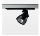
Surface-mounted luminaire with LED, rated life of the LED L80/B10 > 50000 h, colour rendering index CRI > 96, chromaticity tolerance 3 SDCM (initial), reflector with circular light distribution pattern, reflector pure aluminium 99,99% in MIRO-Silver®, rotation angle 330°, swivel angle +85°/-85°, luminaire head/retention arm die-cast aluminium, powder-coated, stratoblack
