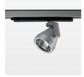
Surface-mounted luminaire with LED, rated life of the LED L80/B10 > 50000 h, colour rendering index CRI > 96, chromaticity tolerance 2 SDCM (initial), reflector with circular light distribution pattern, reflector pure aluminium 99,99% in MIRO-Silver®, rotation angle 330°, swivel angle +85°/-85°, luminaire head/retention arm die-cast aluminium, powder-coated, stratosilver
