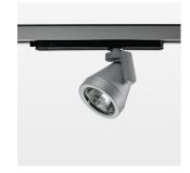
Surface-mounted luminaire with LED, rated life of the LED L80/B10 > 50000 h, colour rendering index CRI > 90, chromaticity tolerance 2 SDCM (initial), reflector with circular light distribution pattern, reflector pure aluminium 99,99% in MIRO-Silver®, rotation angle 330°, swivel angle +85°/-85°, luminaire head/retention arm die-cast aluminium, powder-coated, stratosilver
