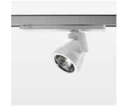
Surface-mounted luminaire with LED, rated life of the LED L80/B10 > 50000 h, colour rendering index CRI > 90, chromaticity tolerance 2 SDCM (initial), reflector with circular light distribution pattern, reflector pure aluminium 99,99% in MIRO-Silver®, rotation angle 330°, swivel angle +85°/-85°, luminaire head/retention arm die-cast aluminium, powder-coated, stratowhite
