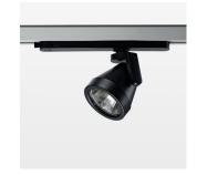
Surface-mounted luminaire with LED, rated life of the LED L80/B10 > 50000 h, colour rendering index CRI > 96, chromaticity tolerance 2 SDCM (initial), reflector with circular light distribution pattern, reflector pure aluminium 99,99% in MIRO-Silver®, rotation angle 330°, swivel angle +85°/-85°, luminaire head/retention arm die-cast aluminium, powder-coated, stratoblack
