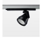
Surface-mounted luminaire with LED, rated life of the LED L80/B10 > 50000 h, colour rendering index CRI > 80, chromaticity tolerance 2 SDCM (initial), reflector with circular light distribution pattern, reflector pure aluminium 99,99% in MIRO-Silver®, rotation angle 330°, swivel angle +85°/-85°, luminaire head/retention arm die-cast aluminium, powder-coated, stratoblack
