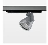
Surface-mounted luminaire with LED, rated life of the LED L80/B10 > 50000 h, colour rendering index CRI > 96, chromaticity tolerance 3 SDCM (initial), reflector with circular light distribution pattern, reflector pure aluminium 99,99% in MIRO-Silver®, rotation angle 330°, swivel angle +85°/-85°, luminaire head/retention arm die-cast aluminium, powder-coated, stratosilver
