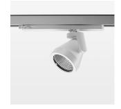
Surface-mounted luminaire with LED, rated life of the LED L80/B10 > 50000 h, colour rendering index CRI > 96, chromaticity tolerance 3 SDCM (initial), reflector with circular light distribution pattern, reflector pure aluminium 99,99% in MIRO-Silver®, rotation angle 330°, swivel angle +85°/-85°, luminaire head/retention arm die-cast aluminium, powder-coated, stratowhite
