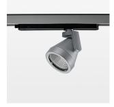
Surface-mounted luminaire with LED, rated life of the LED L80/B10 > 50000 h, colour rendering index CRI > 96, chromaticity tolerance 2 SDCM (initial), reflector with circular light distribution pattern, reflector pure aluminium 99,99% in MIRO-Silver®, rotation angle 330°, swivel angle +85°/-85°, luminaire head/retention arm die-cast aluminium, powder-coated, stratosilver
