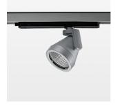
Surface-mounted luminaire with LED, rated life of the LED L80/B10 > 50000 h, colour rendering index CRI > 96, chromaticity tolerance 3 SDCM (initial), reflector with circular light distribution pattern, reflector pure aluminium 99,99% in MIRO-Silver®, rotation angle 330°, swivel angle +85°/-85°, luminaire head/retention arm die-cast aluminium, powder-coated, stratosilver
