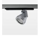
Surface-mounted luminaire with LED, rated life of the LED L80/B10 > 50000 h, colour rendering index CRI > 90, chromaticity tolerance 2 SDCM (initial), reflector with circular light distribution pattern, reflector pure aluminium 99,99% in MIRO-Silver®, rotation angle 330°, swivel angle +85°/-85°, luminaire head/retention arm die-cast aluminium, powder-coated, stratosilver
