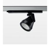
Surface-mounted luminaire with LED, rated life of the LED L80/B10 > 50000 h, colour rendering index CRI > 90, chromaticity tolerance 2 SDCM (initial), reflector with circular light distribution pattern, reflector pure aluminium 99,99% in MIRO-Silver®, rotation angle 330°, swivel angle +85°/-85°, luminaire head/retention arm die-cast aluminium, powder-coated, stratoblack
