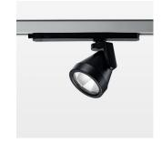
Surface-mounted luminaire with LED, rated life of the LED L80/B10 > 50000 h, colour rendering index CRI > 90, chromaticity tolerance 2 SDCM (initial), reflector with oval light distribution pattern, reflector pure aluminium 99,99% in MIRO-Silver®, rotation angle 330°, swivel angle +85°/-85°, luminaire head/retention arm die-cast aluminium, powder-coated, stratoblack
