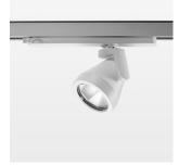
Surface-mounted luminaire with LED, rated life of the LED L80/B10 > 50000 h, colour rendering index CRI > 96, chromaticity tolerance 2 SDCM (initial), reflector with oval light distribution pattern, reflector pure aluminium 99,99% in MIRO-Silver®, rotation angle 330°, swivel angle +85°/-85°, luminaire head/retention arm die-cast aluminium, powder-coated, stratowhite
