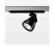
Surface-mounted luminaire with LED, rated life of the LED L80/B10 > 50000 h, colour rendering index CRI > 96, chromaticity tolerance 2 SDCM (initial), reflector with oval light distribution pattern, reflector pure aluminium 99,99% in MIRO-Silver®, rotation angle 330°, swivel angle +85°/-85°, luminaire head/retention arm die-cast aluminium, powder-coated, stratoblack
