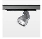
Surface-mounted luminaire with LED, rated life of the LED L80/B10 > 50000 h, colour rendering index CRI > 96, chromaticity tolerance 3 SDCM (initial), reflector with oval light distribution pattern, reflector pure aluminium 99,99% in MIRO-Silver®, rotation angle 330°, swivel angle +85°/-85°, luminaire head/retention arm die-cast aluminium, powder-coated, stratosilver
