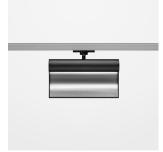
Surface-mounted wallwasher with LED, rated life of the LED L80/B10 > 50000 h, colour rendering index CRI > 90, chromaticity tolerance 3 SDCM (initial), reflector with asymmetrical light distribution pattern, reflector pure aluminium 99,99% in MIRO-Silver®, end caps die-cast aluminium, powder-coated, rotation angle 330°, luminaire housing aluminium extrusion profile, stratoblack
