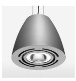
Suspended luminaire with LED, rated life of the LED L80/B10 > 50000 h, chromaticity tolerance 3 SDCM (initial), reflector with circular light distribution pattern, reflector pure aluminium 99,99% in MIRO-Silver®, swivel angle 2x25°, luminaire housing sheet steel, powder-coated, stratosilver
