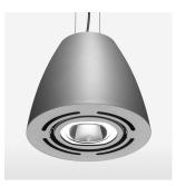
Suspended luminaire with LED, rated life of the LED L80/B10 > 50000 h, chromaticity tolerance 2 SDCM (initial), reflector with circular light distribution pattern, reflector pure aluminium 99,99% in MIRO-Silver®, swivel angle 2x25°, luminaire housing sheet steel, powder-coated, stratosilver
