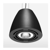
Suspended luminaire with LED, rated life of the LED L80/B10 > 50000 h, colour rendering index CRI > 90, chromaticity tolerance 2 SDCM (initial), reflector with oval light distribution pattern, reflector pure aluminium 99,99% in MIRO-Silver®, swivel angle  $2\times25^\circ$ , luminaire housing sheet steel, powdercoated, stratoblack
