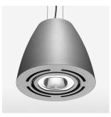
Suspended luminaire with LED, rated life of the LED L80/B10 > 50000 h, colour rendering index CRI > 90, chromaticity tolerance 2 SDCM (initial), reflector with oval light distribution pattern, reflector pure aluminium 99,99% in MIRO-Silver®, swivel angle 2x25°, luminaire housing sheet steel, powder-coated, stratosilver
