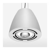
Suspended luminaire with LED, rated life of the LED L80/B10 > 50000 h, chromaticity tolerance 3 SDCM (initial), reflector with circular light distribution pattern, reflector pure aluminium 99,99% in MIRO-Silver®, swivel angle 2x25°, luminaire housing sheet steel, powder-coated, stratowhite
