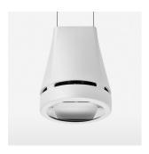
Suspended luminaire with LED, rated life of the LED L80/B10 > 50000 h, chromaticity tolerance 2 SDCM (initial), reflector with oval light distribution pattern, reflector pure aluminium 99,99% in MIRO-Silver®, luminaire head die-cast aluminium, powder-coated, stratowhite, separate driver unit
