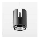
Suspended luminaire with LED, rated life of the LED L80/B10 > 50000 h, colour rendering index CRI > 80, chromaticity tolerance 2 SDCM (initial), LED hybrid technology, 3D silicone lens to reduce the proportion of scattered light, reflector with oval light distribution pattern, reflector pure aluminium 99,99% in MIRO-Silver®, segmented, exchangeable reflector unit in high-sheen black plastic, with glass cover, luminaire housing die-cast aluminium, powder-coated, stratoblack, separate driver unit
