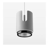
Suspended luminaire with LED, rated life of the LED L80/B10 > 50000 h, chromaticity tolerance 2 SDCM (initial), LED hybrid technology, 3D silicone lens to reduce the proportion of scattered light, reflector with oval light distribution pattern, reflector pure aluminium 99,99% in MIRO-Silver®, segmented, exchangeable reflector unit in high-sheen black plastic, with glass cover, luminaire housing die-cast aluminium, powder-coated, stratosilver, separate driver unit
